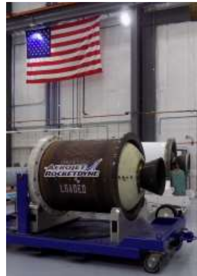
Figure 6. The eSR-73 was a successful pathfinder for the transition of our large SRM manufacturing capabilities to our Camden, AR facility.
